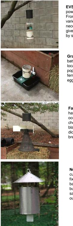
**EVS (Encephalitis virus surveillance) trap.** This trap is powered by 3 D-cell batteries in a plastic pvc 'flashlight' tube. From 20-40 of these are operated weekly for 24 hour periods in various locations where spot checks of mosquito populations are necessary. The black can contains a chunk of dry ice which gives off carbon dioxide as it evaporates, attracting mosquitoes by simulating the breath of an animal or human.
